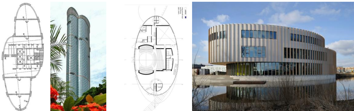
Figure 12: The 73 stories Highcliff Apartments Building in Hong Kong (left) and the Bijlmer Park Theater in Amsterdam (right) are examples of juxtaposed ellipses.
